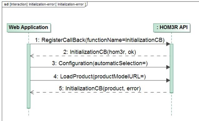
Figure 13: Sequence diagram of an initialization and load of models scenario with errors
