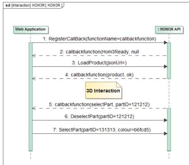
Figure 14: Sequence diagram showing an example of the interface interaction. The web application registers a callback function and asks HOM3R to start the product model load. During interaction, HOM3R uses the callback to inform the web application that a part has been selected by the user and the web application requests HOM3R to unselect that part and select a new one
