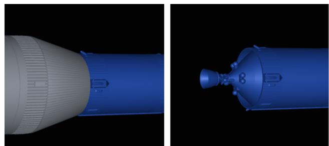
Figure 6: Example of parts removal. Left: the selected part, in blue, is not fully visible. Right: the user has manually removed the occluding parts in order to visualize the selection complete
