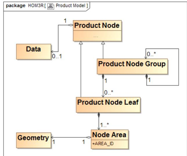
Figure 2: Simplified product model class diagram
