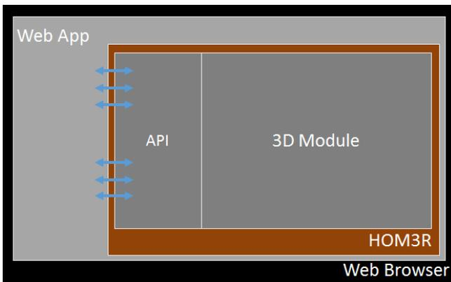
Figure 10: High-level architecture block diagram of HOM3R
