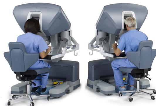
Figure 3: Multi-user telesurgery system: both surgeons are able to control the surgical system at the same time and over large distances. © 2014 Intuitive Surgical, Inc.
