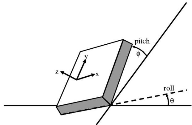
Figure 1: Compass tilt referenced to horizontal plane
