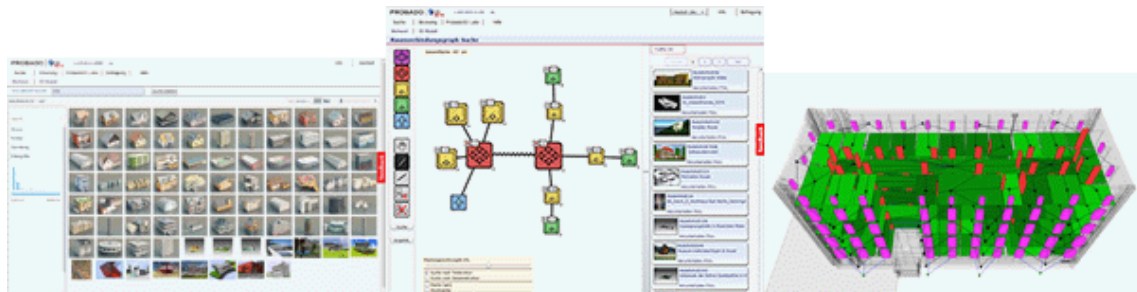
Fig. 1. The Probado 3D Webinterface for query formulation and result presentation [1]: Faceted search (left); Query with spatial configuration of rooms (middle); Building with Room Connectivity Graph (right).
